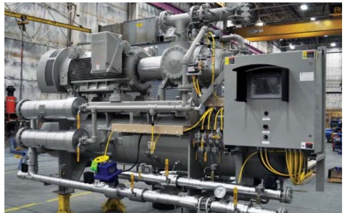
Vilter Single Screw propane refrigeration unit, destined for new Oklahoma gas processing plant.
